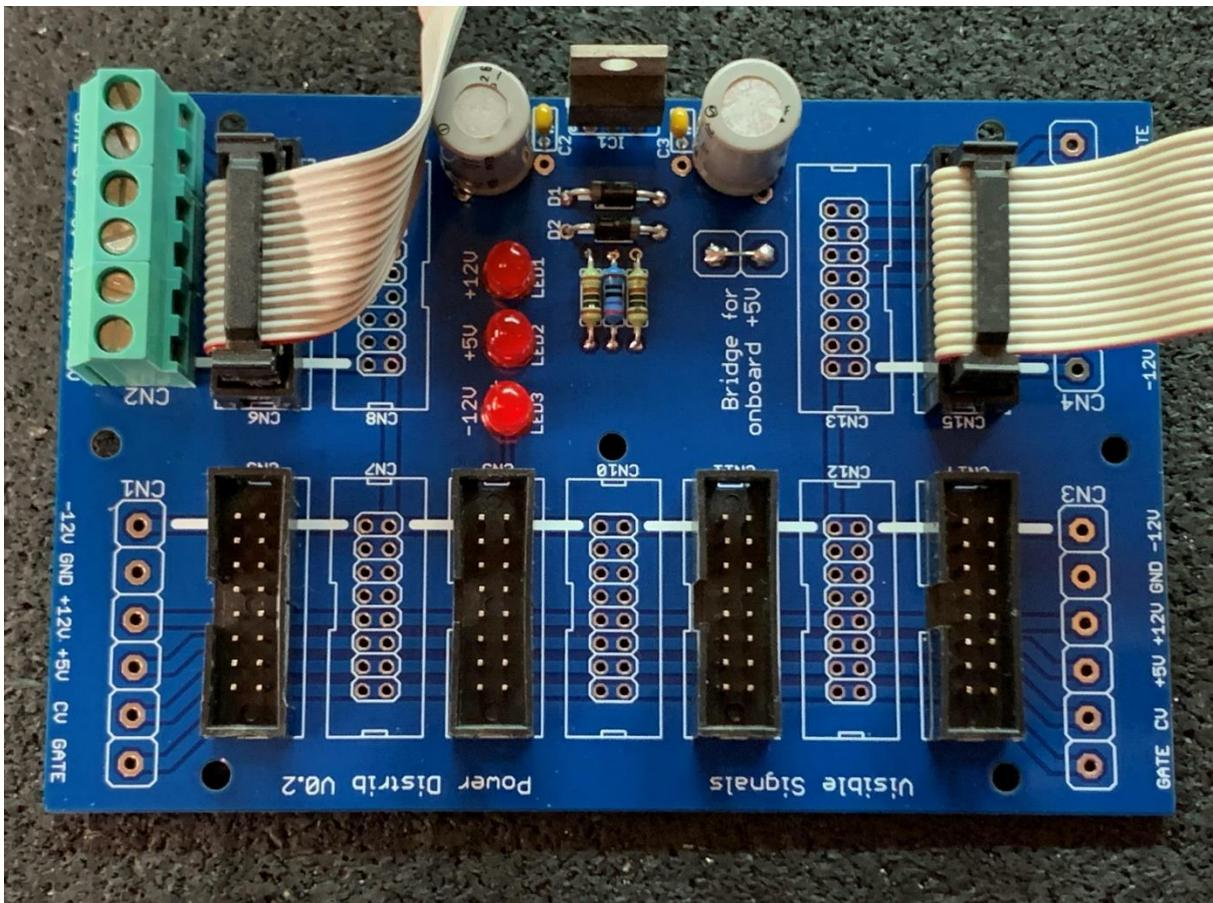
Power Distrib is a bus board for power distribution in a eurorack modular system. It features eleven 16-pin power connector sockets, an optional on-board +5V regulator, power rail indicator LEDs and four heavy-duty screw or solder-type connection points to support star or chained power distribution topologies.
