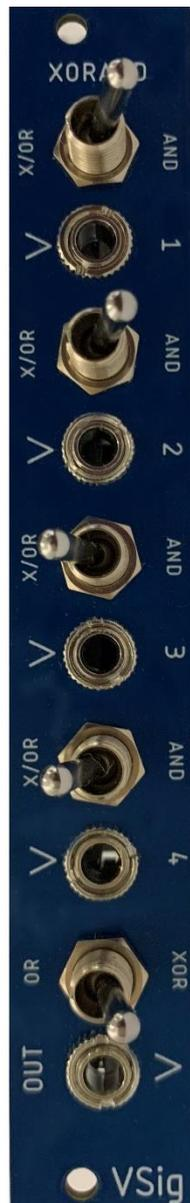
Xorand is a 4HP four-input logic gate performance control module for LZX-compatible eurorack video module systems.
