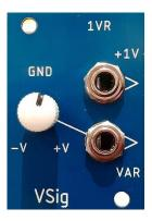
1VR Voltage Rererence is a 6HP 1U tile which provides two stable voltage references suitable for video use: +1V (fixed) and -1V to +1V (adjustable).
