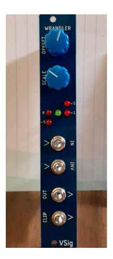
The Wrangler is voltage processing module designed for manipulating and monitoring video synth control voltages. It features a two-input video signal mixer (one of which is normally inverted), panel controls for voltage offset and scaling to allow conversion to and from conventional Eurorack +/-12V signal levels, a five-LED level meter to indicate the output voltage signal, and two buffered outputs (one with 0 to 1V video-range clipping).
